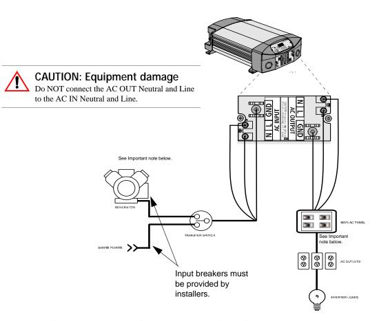
Figure 1-7 AC Wiring Diagram without an Inverter Subpanel
