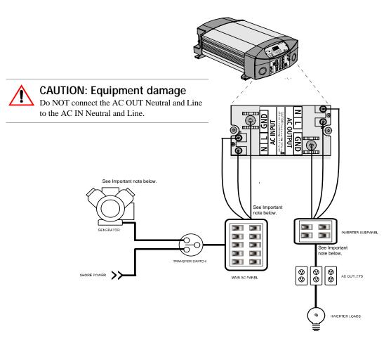
Figure 1-6 AC Wiring Diagram with an Inverter Subpanel
