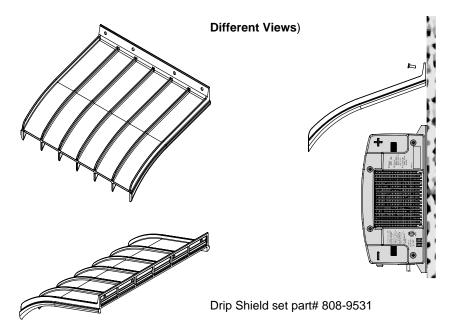
Figure 1-10 Drip Shields
