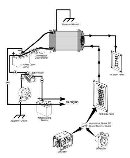
Figure 1-2 Typical Recreational Vehicle and Fleet Vehicle Installation
